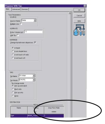
Figure 2: 735 Sampler Software Task Used to Dispense the Sample into the E-Gel® 96 gels Variables (#volume) can be used if different volumes of sample are required and can be imported via a Microsoft® Excel® spreadsheet.
