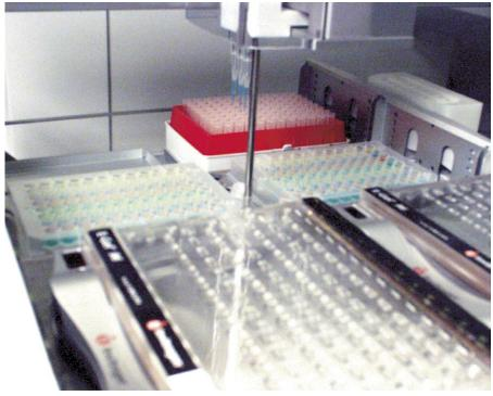
Photo 4: Quad-Z 215 with Disposable Tips Demonstrating Independent Tip Movement Independent tip movement allows the Quad-Z 215 with Disposable Tips to access a single vial.
