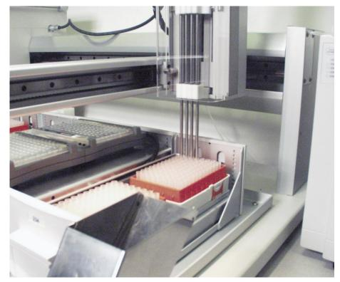
Photo 2: Quad-Z 215 Picking Up 10-µL Disposable Tips Prior to Sample Aspiration
