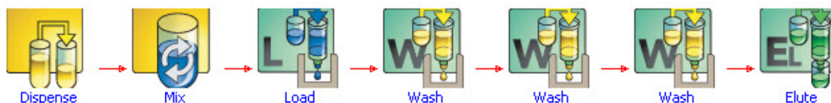
Figure 5. TRILUTION® LH Solid Phase Extraction Method Using the GX-274 System
