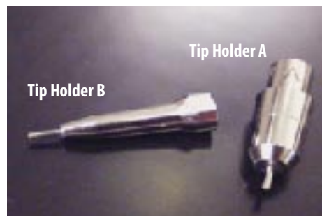
Photo 5: Tip Holder Styles for the Quad-Z 215 with Disposable Tips
