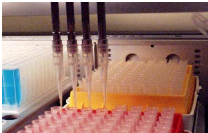
Photo 3: Quad-Z 215 with 10- \mu L Disposable Tips
