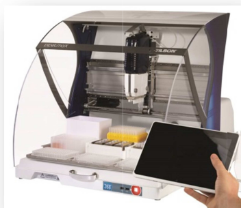
Figure 1. PIPETMAX Normalization Assistant.
