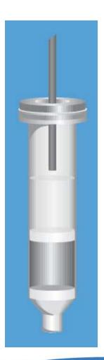
The probe introduces the sample or solvent to the SPE cartridge, once delivery is complete a gas valve is turned on by the software and Nitrogen is introduced to the cartridge which pushes the liquid through the cartridge. The time that the cartridge is exposed to the gas pressure is settable, hence **DRYING or NOT DRYING the** cartridge is not an issue and since every cartridge is treated exactly the same, consistency is optimized from the 1st cartridge to the last cartridge.
