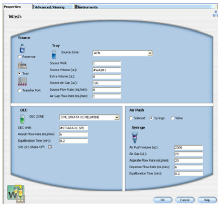
Figure 3. Wash Task Page in TRILUTION LH Method Builder. The open fields for all method tasks allows for easy method development with no manual intervention.
