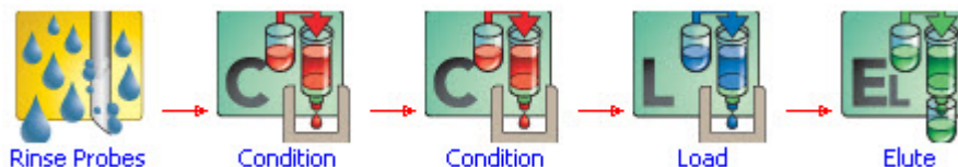
Figure 2. TRILUTION LH SPE Tasks for Extraction of Sucralose from Water
