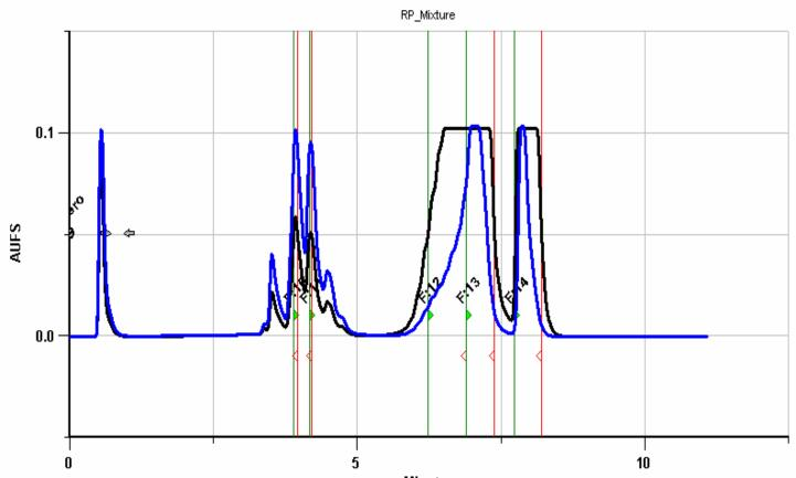
The above RP chromatogram represents the chromatography established for a mixture of three components (Caffeine 102 mgs, p-hydroxy benzoic acid ethyl ester 68 mgs, biphenyl 69 mg: total on column injection of 239 mg in a 4 mL injection volume. A gradient 5-95% Water:ACN was run over 7 minutes. Fractions collected were injected under analytical conditions to determine the components of the fractions collected.
