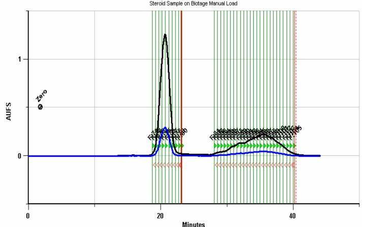
The above NP chromatogram was produce from the Biotage FLASH 40+M column. The column was manually loaded with 15 mls of solution (THF/Dioxane) in which 445 mg of sample was dissolved (Estrone: 318 mgs and Estriol 127 mgs), flow rate of 30 mls/min, Hexane/IPA (90:10)
