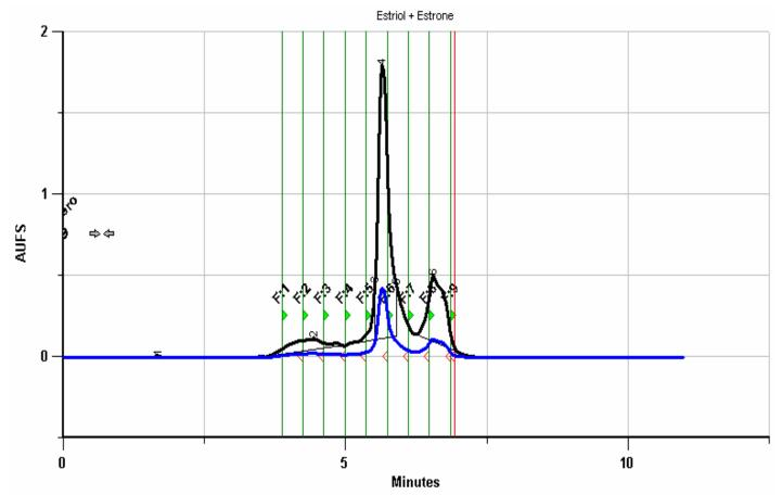
The above NP chromatogram was achieved with a Betasil silica column 20x150 mm, 5µ, 100A. The sample (156 mg) was Estrone (96 mg) and Estriol (60 mg) in a 4 mL injection on column. An isocratic run of Hexane/IPA (98:2) chromatographed the sample in less than 10 minutes.
