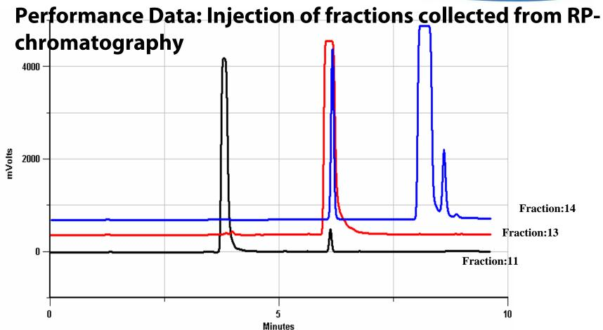
Fractions collected from RP-CombiPrep column were injected without dry down on-line onto an analytical system. The samples were run on a Sulpelco 4.6x 150 mm, 5  $\mu$ , 100A, 1.5 mL/min, 5-95% Water:Acetonitrile over 7 minutes, 40 uL of each fraction was injection onto the column. The overlay shows the separation of the three components that were injected onto the semi-preparative column and fractions collected.
