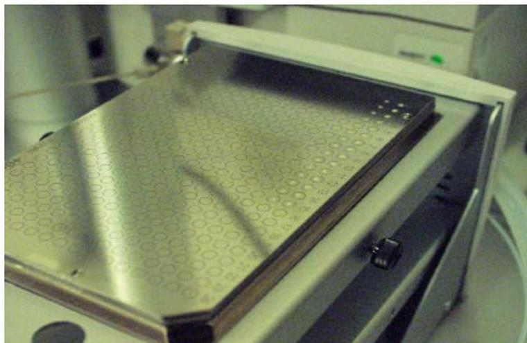
**Photo 1: Bruker AnchorChip™ Plate with Matrix Spotted via the Spring-Loaded Probe (1 and 0.5  $\mu$ L, respectively)**
