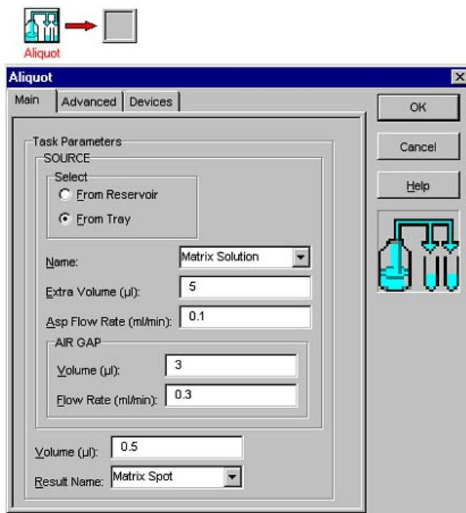
**Figures 3 & 4: 735 Tray File and Method for the MALDI Spotting of the Matrix**
