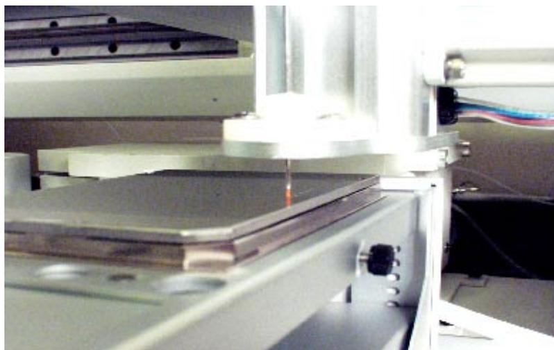
**Photo 2: Side View of the Spring-Loaded Probe (on the Micro 215) Spotting the MALDI Plate**
