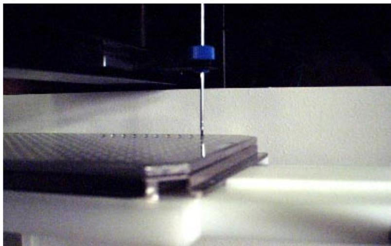
**Photo 3: Fraction Collection onto the MALDI Plate with the Spring-Loaded Probe (on the 223 Liquid Handler)**
