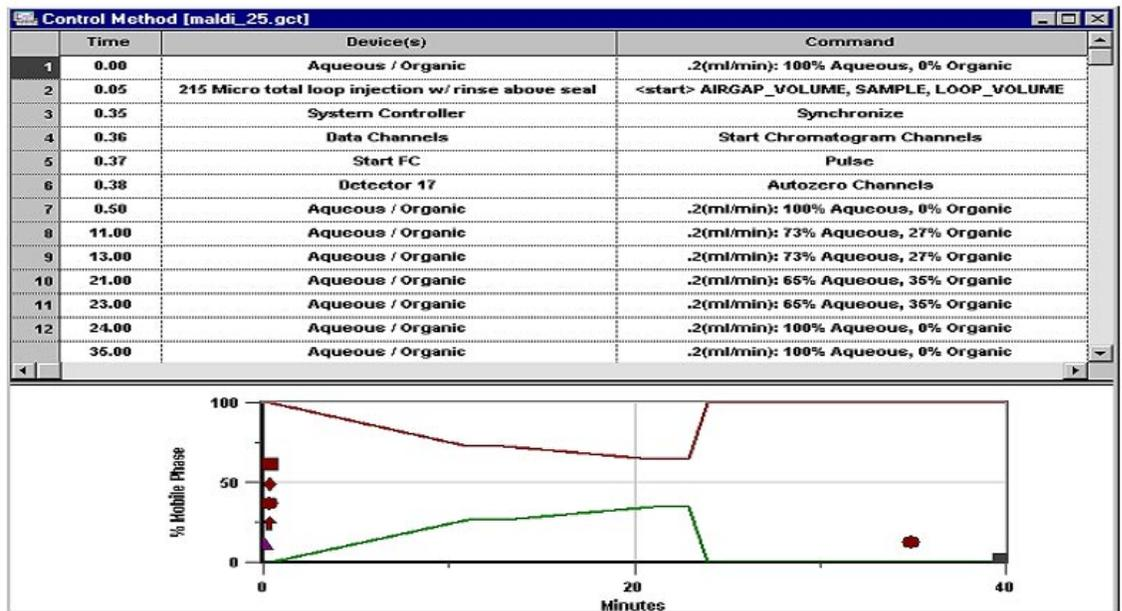
The system was run at 0.2 mL/min. with the splitter set to achieve a flow rate of 6  $\mu$ L/min. through the capillary column.
