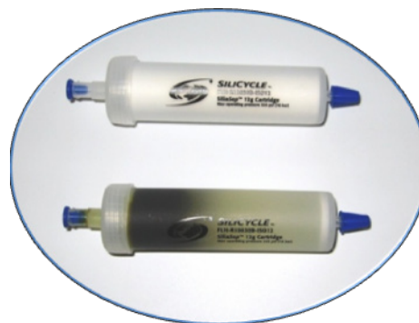
Figure 4. Silica flash cartridge before and after tea extract injection.
