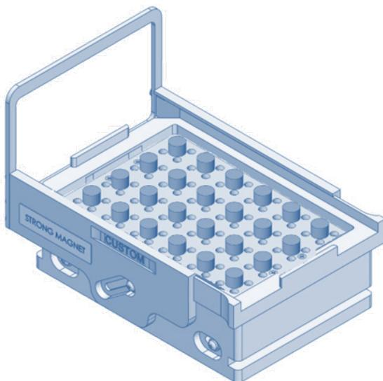
**Figure 2:** The custom magnetic bead separator (part number SPL2294) contains 24 magnets which can be raised or lowered to be in close contact with a 96 well plate. Each magnet is positioned between four wells, pulling the magnetic beads to the corner of each well.
