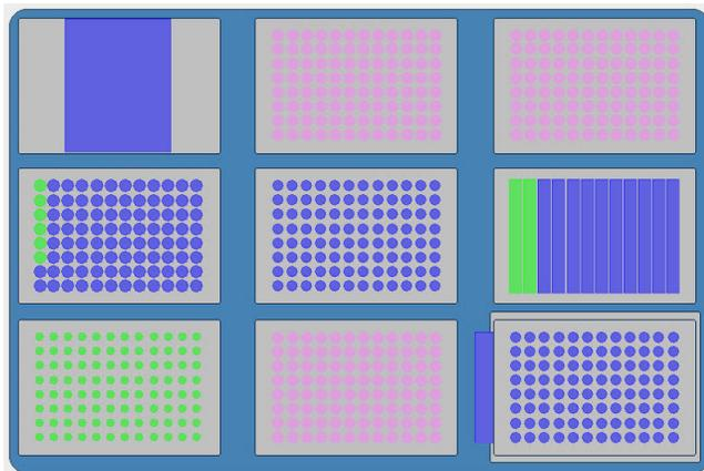
**Figure 4:** User interface for bed layout on PIPETMAX®. Labware and reagents from left to right, back to front: Tip Waste Chute, DSF200ST Tip Rack, DSF200ST Tip Rack, RSB Resuspension buffer in 0.2mL 8-Tube Strips, empty MIDI plate for final eluted libraries, liquid reservoir containing AMPure® XP beads and 80% Ethanol, starting material (amplified Libraries, DSF200ST Tip Rack, and another empty MIDI plate on the magnetic bead separator for the clean-up procedure.
